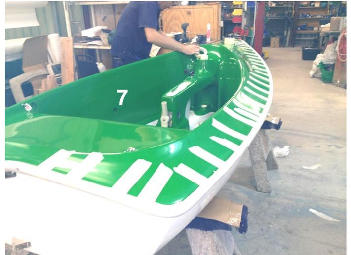
8. Clean off excess with acetone of turps and small rags. Better to cut and tear rags into small pieces and discard them, rather than a big rag which spreads the adhesive everywhere. After initial clean, particularly on the underside, press strip home again checking it is pushed onto the hull surface, that its correctly wrapped under the flange, then apply masking tape, wrapped underneath and taped onto the deck about every 150mm to keep it in place.
