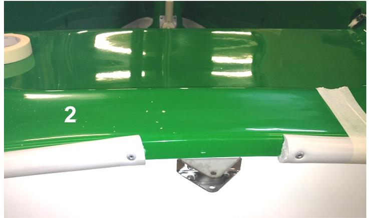
3. Remove, coil up and place in heating box for about 30 minutes till evenly pliable, which is around 60 degrees.
