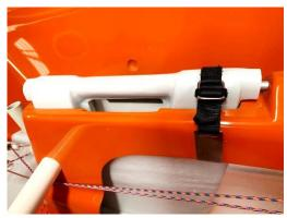
be sailing solo in fleet racing, or in violent and changeable wind conditions. There will also be occasions where the keel handle tube is damaged restricting the long pin. Well you need to fix this ASAP, but to lock down the keel in the short term the secondary lock down strap will keep the keel in place.
