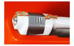
2. The shock cord strop is a very simple device which ensures the long pin remains inserted with about 50mm into the fibreglass console. We have seen boats lifted clear of the water when in the process of removing the keel with a C Crane, they forgot to first remove the long pin. In this situation the further the long pin inserts into the console the
