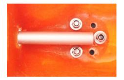
Above are 2 photos taken underneath the console looking up at the cleat fastenings. The photo on the right shows the Ronstan cleat swivel rotated 180 degrees so the fully inserted 430mm Long Pin passes underneath. Fully inserted means Pin followed by cord and knot, or the cork.
